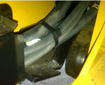
Supertrak is proud to offer an Industry First Hydraulic Hose Guard Kit for your Caterpillar® C-Series MTL/CTL Models. The Hose Guard Kits provides protection of the Drive motor lines in applications like Forestry, Recycling.
